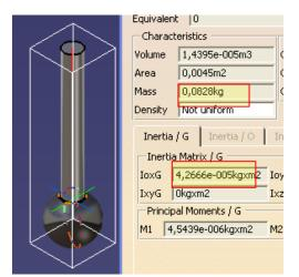
Fig. 4. Estimation of the moment of inertia about the centre of mass **J**<sub>\*</sub> using CAD software
